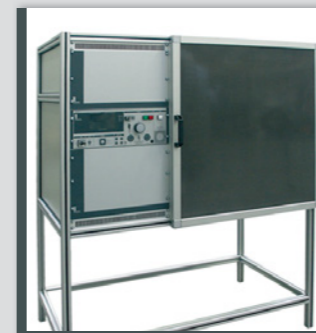
High-voltage test station up to 40KV
