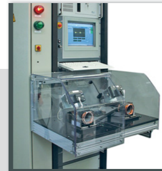
Dual station with MTC3 in 19"-cabinet
