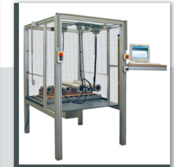
Large test cage with conveyor belt, light curtain and side doors with pneumatic control
