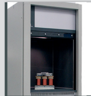
High-voltage test station up to 20KV for electronic modules
