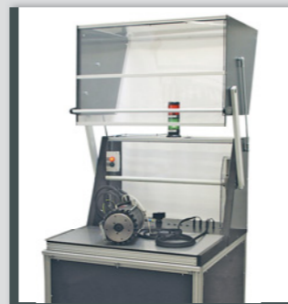
This test cover can be opened and closed easily and remain in any desired position
