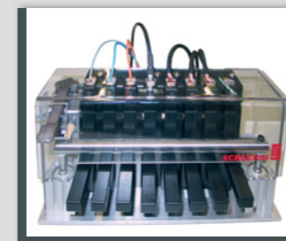
Block with Kelvin clamps with automatic release
