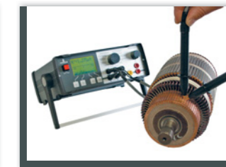
Resistance test at an armature between the lamellas
