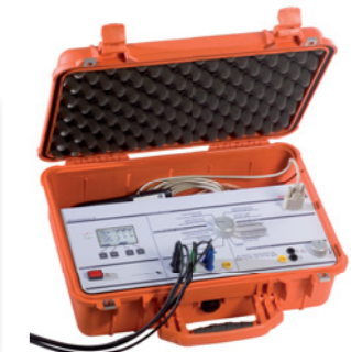
MotorAnalyzer in measurement case suitable as hand luggage
